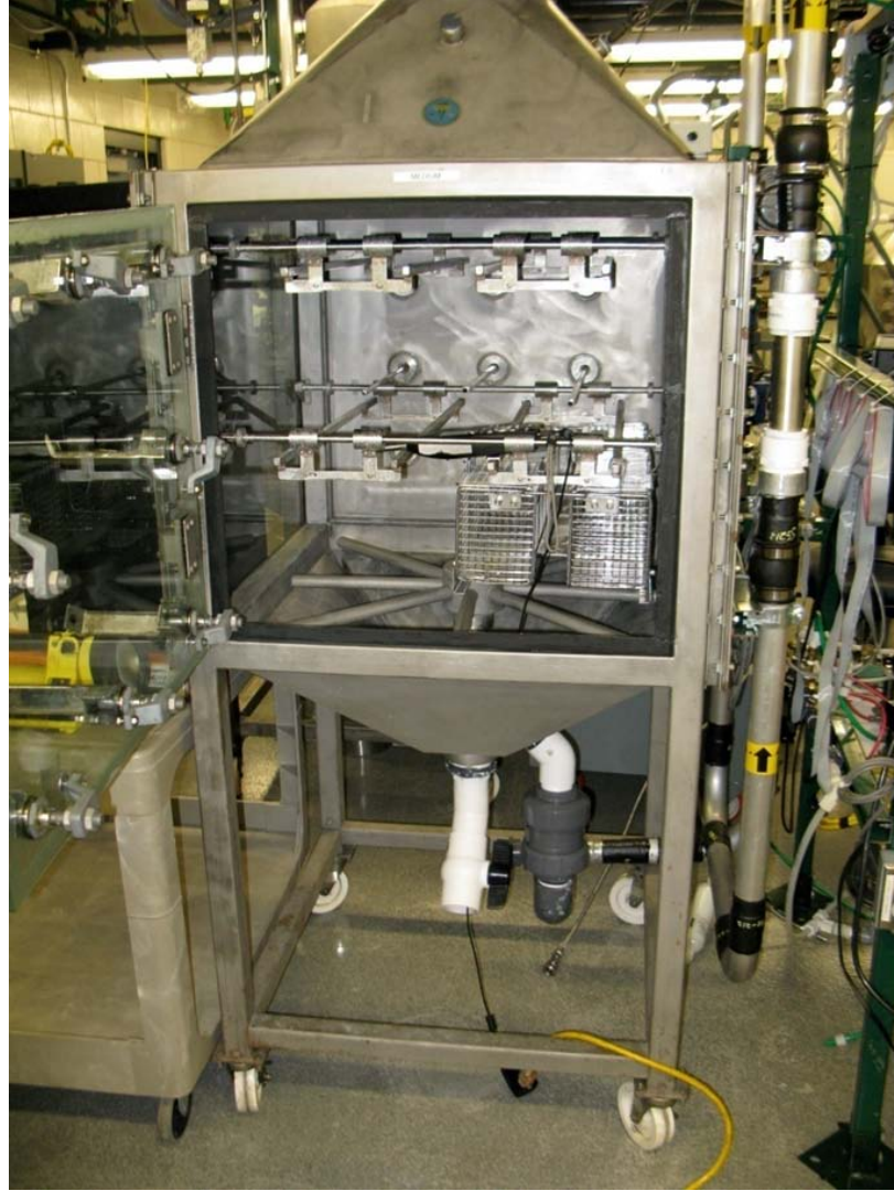
Figure 4. Whole body aerosol exposure chamber
