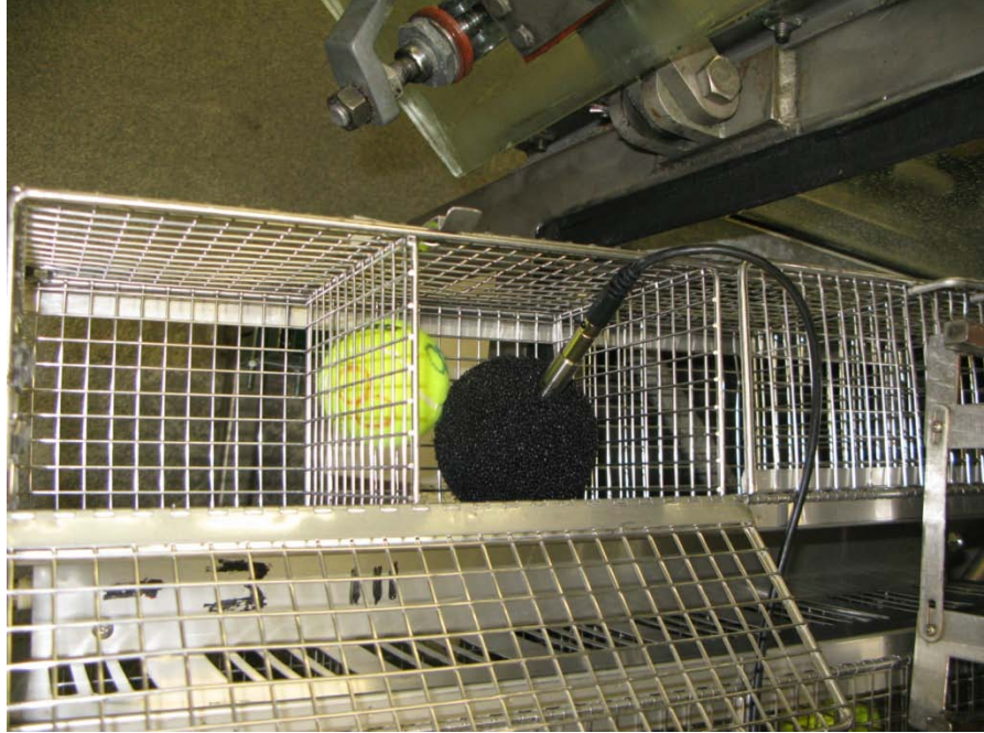
Figure 11. Microphone positioned with windscreen within a cage assembly
