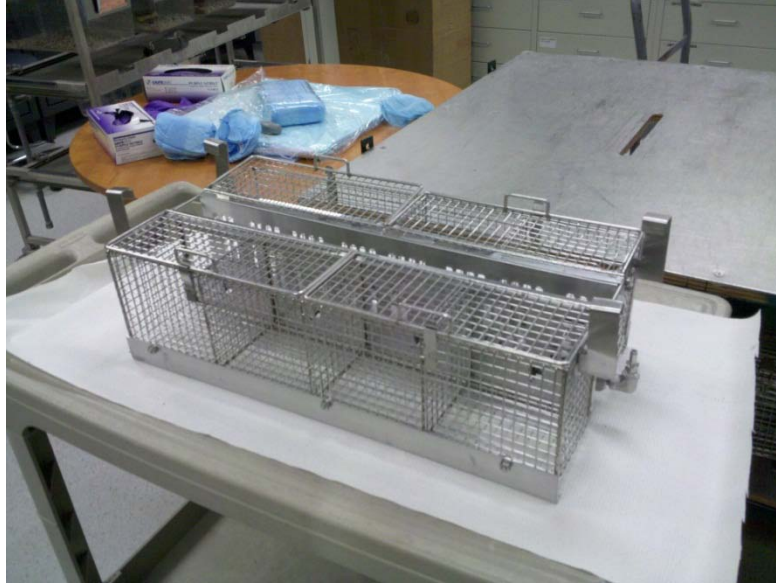
Figure 5. Cage assembly with eight individual compartments
